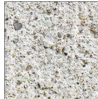
LIGHT SANDBLAST AGGRIGATED TILT WALL CONCRETE EXAMPLE
