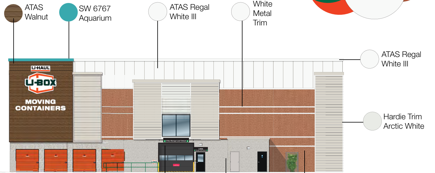
SOUTH ELEVATION - BLDG. B
