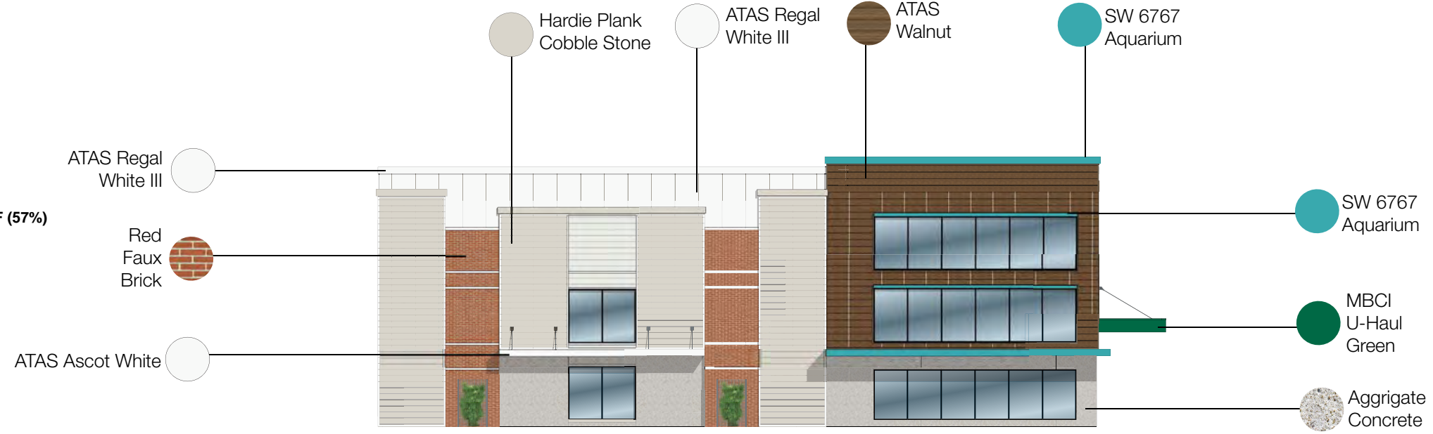
WEST ELEVATION - BLDG. A
