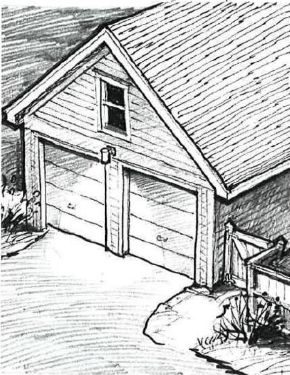
Along alleys, a simple wall-mounted down-light, controlled by a photocell and timer, provides adequate lighting without creating a nuisance.
