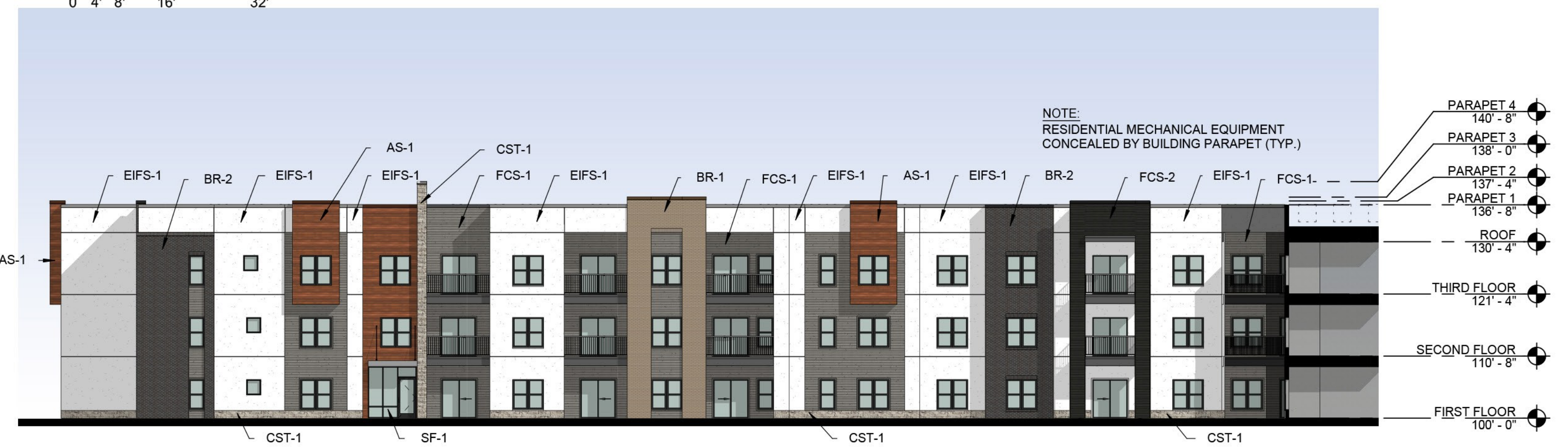
3 SOUTH ELEVATION (W)
