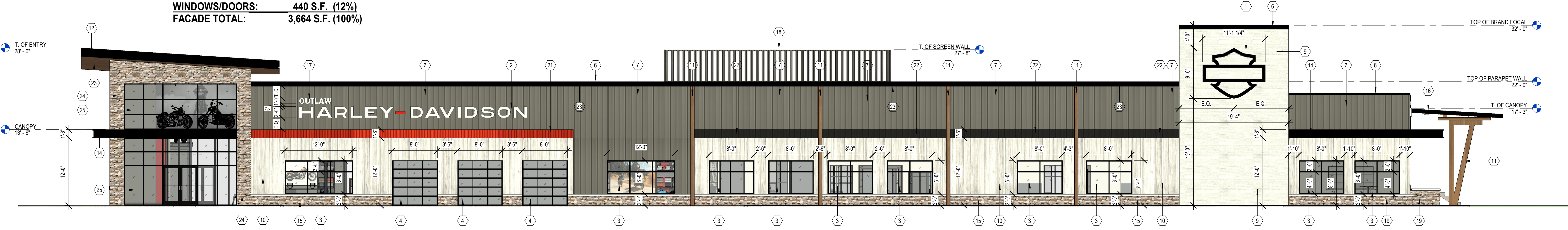
2 SOUTH ELEVATION SCALE: 1/8" = 1'-0" METAL PANELS: 1,739 S.F. (33%) FAUX FIBER CEMENT: 1,634 S.F. (32%) THIN STONE VENEER: 545 S.F. (11%) WINDOWS/DOORS: 1,260 S.F. (24%) FACADE TOTAL: 5,178 S.F. (100%)
