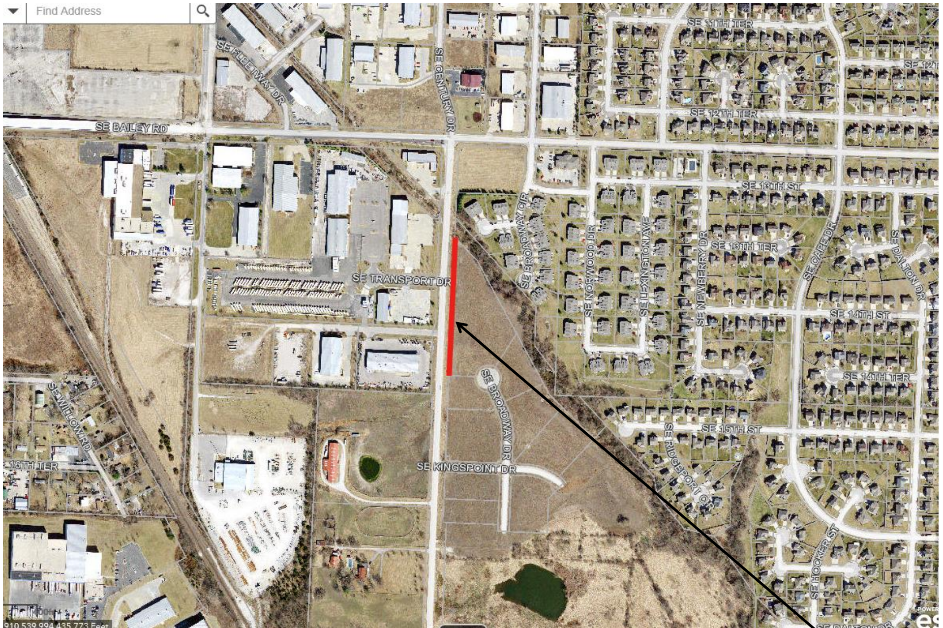
HT Solutions – 1440 SE Broadway Dr. – map of area where 5' public sidewalk is required for the project (approx. 730')
