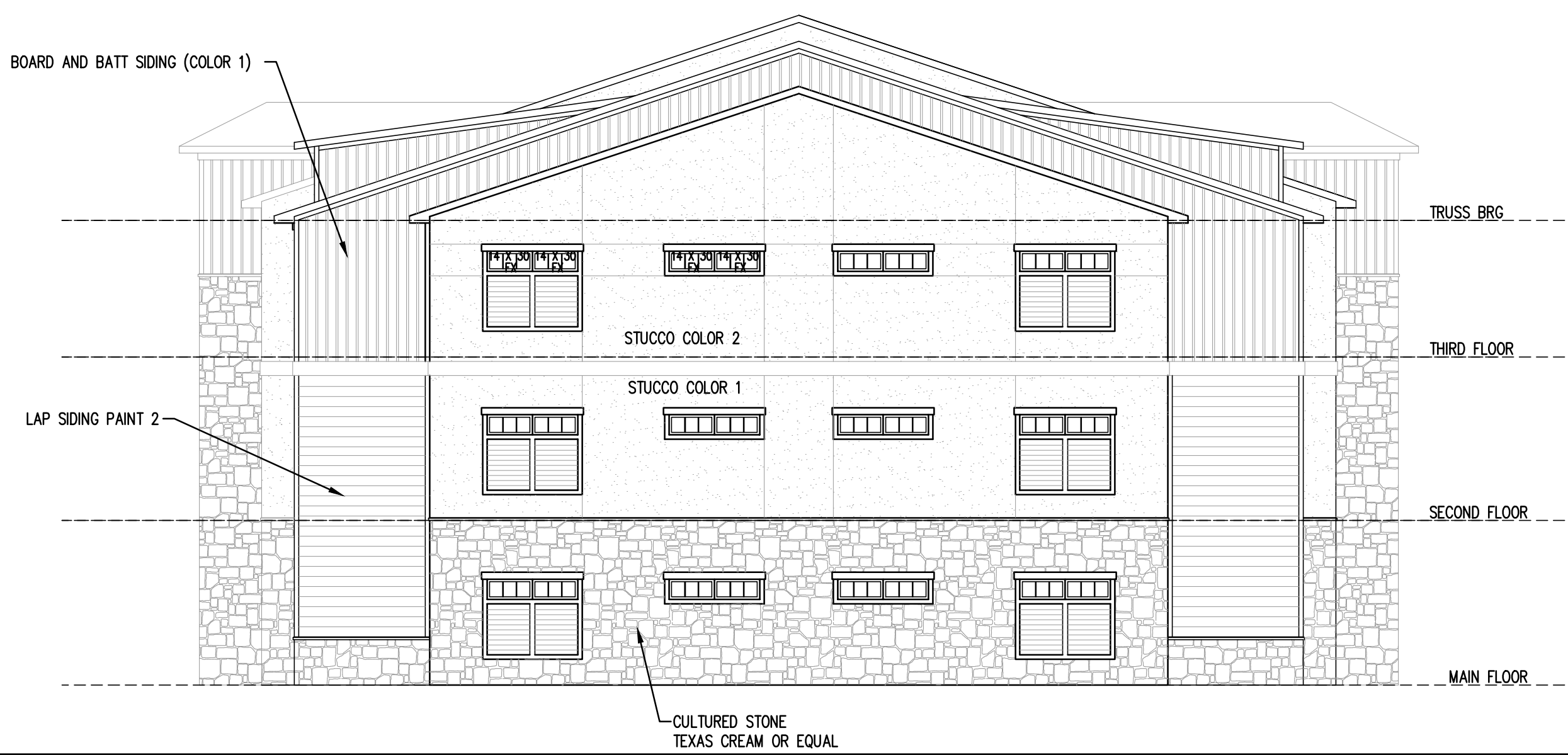
4 BUILDING C1-1 WEST ELEVATION 1/8" = 1'-0"
