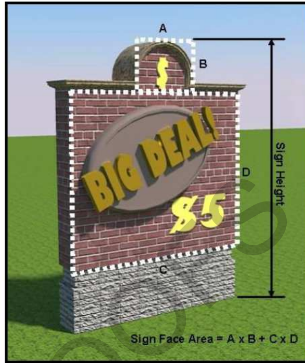
Measuring Sign Face and Sign Height
