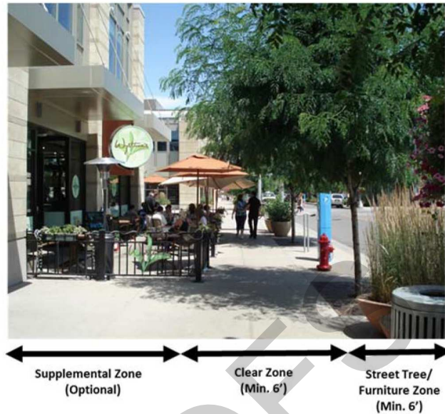
Figure 5.510.B-19: Delineation of Sidewalk Area
