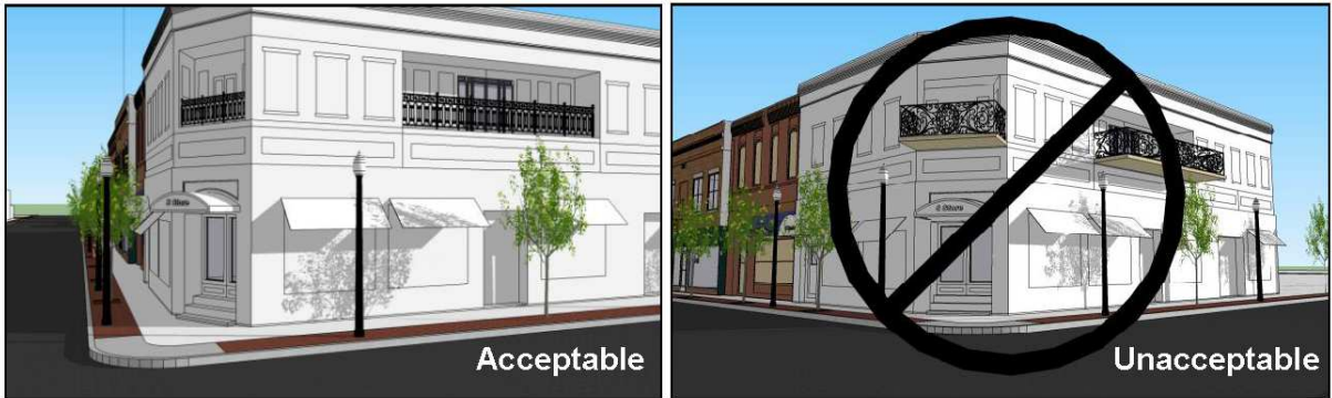
Upper story balconies on the front of buildings must be recessed, not projecting.
