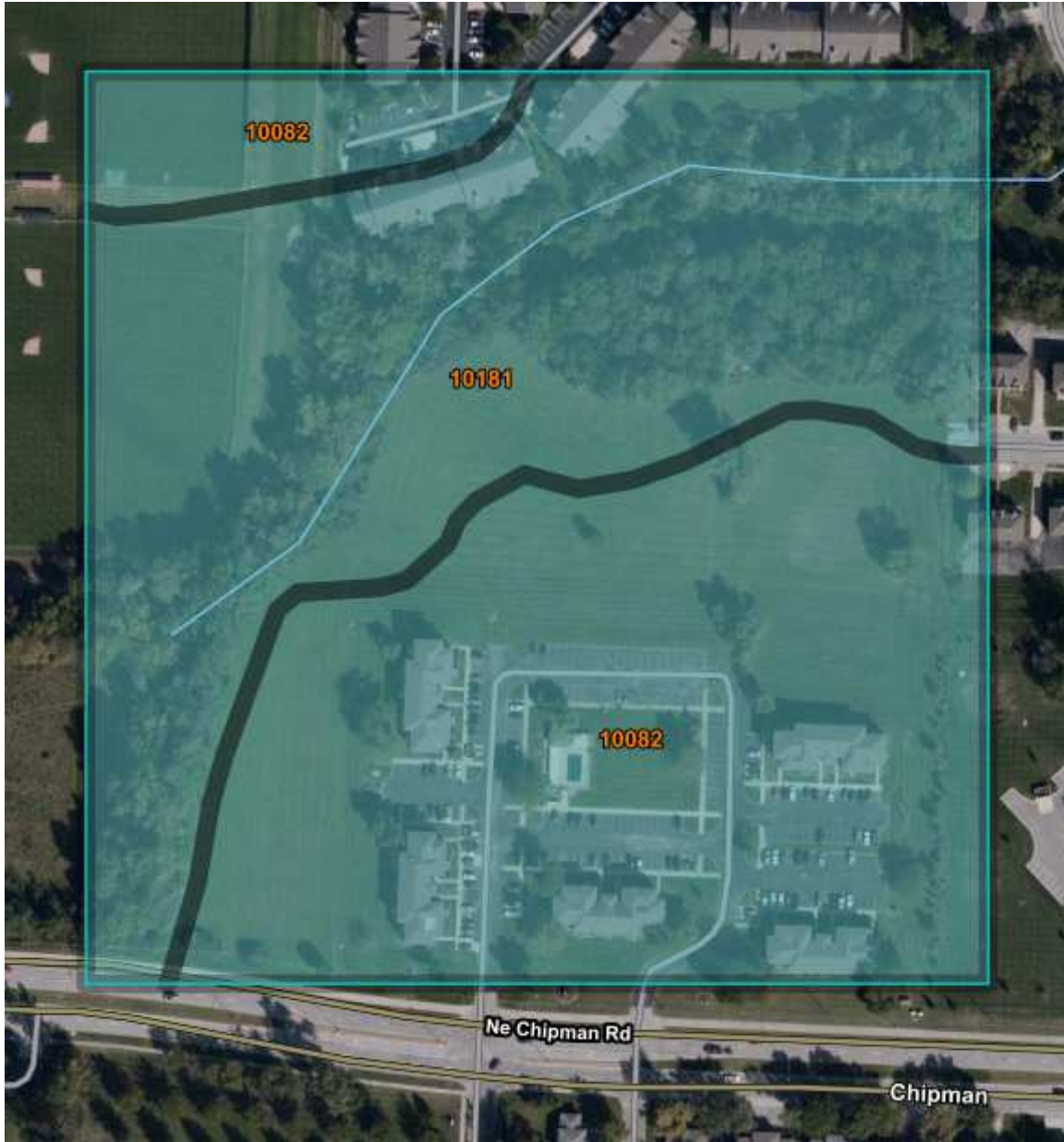
NRCS Web Soil Survey Map of the Summit Point Apartments (Blue shading indicates Type-C Soils)
