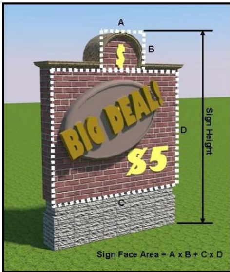
Measuring Sign Face and Sign Height
