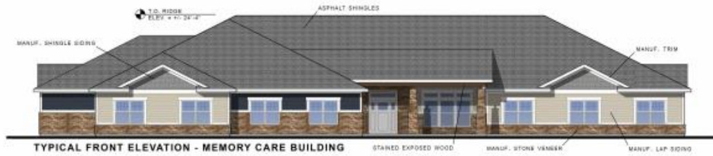
TYPICAL FRONT ELEVATION - MEMORY CARE BUILDING
